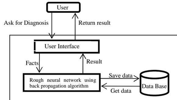
Figure2. System architecture
